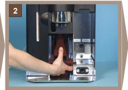
Reach into the brewer area under the brewing unit with one hand and release the retaining catch.
